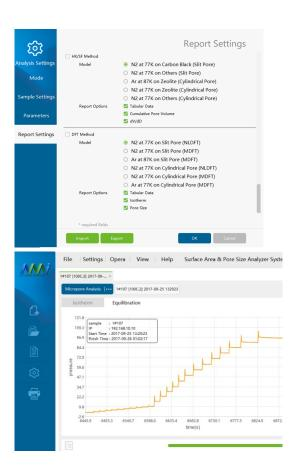
PAS Software adopts a unique doing control method, the pressure in adsorption and desorption process is optimally set in six-stages.
